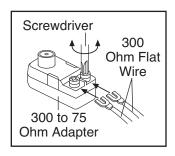
Push the 300 ohm to 75 ohm adapter onto the 75 ohm terminal on the treadmill frame near the power cord.
